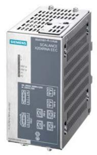
Configurable version for use in PRP or HSR networks SCALANCE X204RNA EEC; redundant network access 2x 100 Mbit/s RJ45 ports; 2x 100 Mbit/s combo ports; LED diagnostics; error signaling contact with set button; simple power supply; network management; incl. electronic manual on CD-ROM, C-plug optional for PRP and HSR networks;
