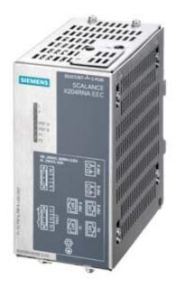
SCALANCE X204RNA EEC; redundant network access 2x 100 Mbit/s RJ45 ports; 2x 100 Mbit/s combo ports; LED diagnostics; error signaling contact with set button; simple power supply; network management; incl. electronic manual on CD-ROM, C-plug optional for PRP network
