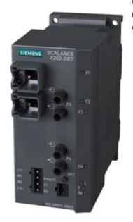
SCALANCE X202-2IRT managed IE IRT switch, 2x 10/100 Mbit/s RJ45 ports, 2x 100 Mbit/s Multimode BFOC, Error signaling contact with set button, Redundant power supply, PROFINET IO device, network management, Redundancy Manager integrated, incl. electron. manual on CD-ROM, C-plug optional
