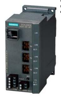
SCALANCE X201-3PIRT managed IE IRT switch, 1x 10/100 Mbit/s RJ45 ports, 3x 100 Mbit/s POF SC RJ ports, Error signaling contact with set button, Redundant power supply, PROFINET IO device, network management, Redundancy Manager integrated, incl. electron. manual on CD-ROM, C-plug optional
