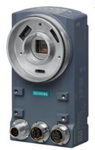
SIMATIC MV560 U optical reader Resolution: 1920 x 1200 pixels; Maximum processing and communication speed; Function: 1D/2D code reading; Image field and distance: variable, (lens); PoE; IP67 with 6GF3540-8AC12; Delivery: reader; B enable => VS enable
