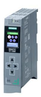
SIMATIC S7-1500T, CPU 1511T-1 PN, central processing unit with working memory 225 KB for program and 1 MB for data, 1. interface: PROFINET IRT with 2 port switch, 60 ns bit performance, SIMATIC memory card necessary
