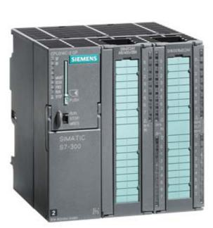
SIMATIC S7-300, CPU 314C-2 DP Compact CPU with MPI, 24 DI/16 DO, 4 AI, 2 AO, 1 Pt100, 4 high-speed counters (60 kHz), integrated DP interface, Integr. power supply 24 V DC, work memory 192 KB, Front connector (2x 40-pole) and Micro Memory Card required
