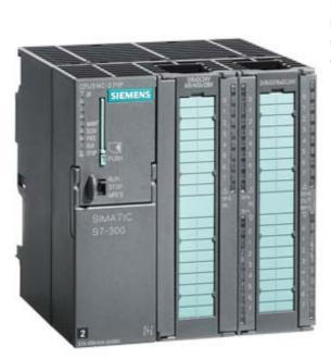
SIMATIC S7-300, CPU 314C-2 PTP Compact CPU with MPI, 24 DI/16 DO, 4 AI, 2 AO, 1 Pt100, 4 high-speed counters (60 kHz), integrated interface RS485, Integr. power supply 24 V DC, work memory 192 KB, Front connector (2x 40-pole) and Micro Memory Card required
