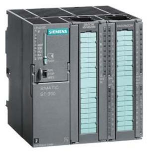
SIMATIC S7-300, CPU 313C, Compact CPU with MPI, 24 DI/16 DO, 4 AI, 2 AO, 1 Pt100, 3 high-speed counters (30 kHz), Integr. power supply 24 V DC, work memory 128 KB, Front connector (2x 40-pole) and Micro Memory Card required
