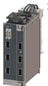
SIPLUS HCS4300 POM4320 Busbar mounting (IEC). Power output module for mounting on busbars system. Redesign with increased interference immunity. With 9 outputs each max. 7680 W (for operating mode Half-wave control: Depending on the Inrush current of the load limitation to max. 4000 W)
