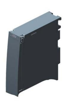
SIPLUS S7-1500 CM PTP RS 422/485 TX rail -40...+70°C TX with 85°C for 10 minutes with conformal coating based on 6ES7541-1AB00-0AB0 . Communication module for serial connection RS 422 and RS 485, Freeport, 3964 (R), USS, MODBUS RTU master, slave, 115200 Kbit/s, 15-pin D-sub socket
