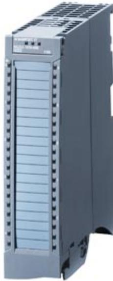
SIPLUS S7-1500 AI 8xU/I/RTD/TC TX RAIL -40 ... +70°C T1 with 85°C for 10 min with conformal coating based on 6ES7531-7KF00-0AB0 . analog input module AI 8 X U/I/RTD/TC ST, 16 bits of resolution, "accuracy 0.3 %; 8 chnnels in" "groups of 8; 4 channels for RTD" measuring, COMMON MODE VOLTAGE "APPR. 10 V; DIAGNOSIS," PROCESSALARMS INCL. INFEEED ELEMENT, SHIELD CLAMP AND SHIELD TERMINAL
