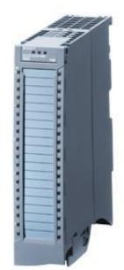
SIPLUS S7-1500 DI 16x110VDC HF TX RAIL -40 ... +70°C TX with 85°C for 10 min with conformal coating based on 6ES7521-7EH00-0AB0 . DI 16x24 ... 125V UC HF, 16 channels in groups of 1 Input delay 0,05 ... 20ms Input type 3 (IEC "61131); diagnostics, Hardware" interrupts
