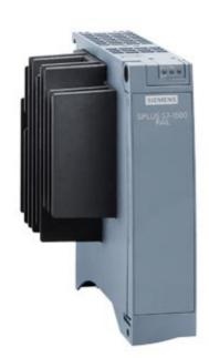
SIPLUS S7-1500 CPU 1511-1 PN TX RAIL -40 ... +70°C TX with 85°C for 10 min with conformal coating based on 6ES7511-1AK01-0AB0 . Central processing unit with RAM 150 KB for program and 1 MB for data, 1st interface: PROFINET IRT with 2-PORT SWITCH, 60 ns bit performance, SIMATIC Memory Card required without display
