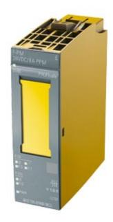
SIPLUS ET 200SP F-PM-E 24 V DC/8A PPM RAIL -25 ... +55°C T1 with 70°C for 10 min with conformal coating based on 6ES7136-6PA00-0BC0 . POWER M. F-PM-E PPM PROFIsafe, for ET "200SP; 24 V DC safe shutdown of" DQ and F-DQ up to PL D/SIL2 or PL E/SIL3 2 safe dig. inputs 1 safe dig. output PPM
