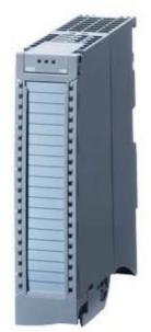
SIPLUS S7-1500 AQ 8xU/I HS -40...+70 °C Start up -25 °C with conformal coating based on 6ES7532-5HF00-0AB0 . Analog output module AQ8xU/I HS, 16 bit resolution, Accuracy 0.4%, 8 channels in groups of 8, "diagnostics; substitute value" 8 channels in 0.125 ms incl. infeed element, Shield bracket and shield terminal
