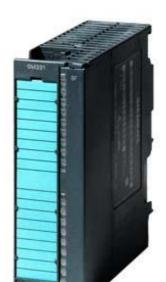
SIPLUS S7-300 SM 331 8AI 40-pole with conformal coating based on 6ES7331-7PF11-0AB0. Analog input isolated, 8 Al thermocouples Type B, E, J, K, L, N, R, S, T TXK/TXK (L) according to GOST 16 bit, 50ms, 1x 40-pole
