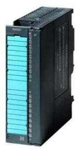
SIPLUS S7-300 SM 331 8AI with conformal coating based on 6ES7331-7PF01-0AB0 . Analog input isolated, 2/3/4-wire, 8 Al, Resistor, Pt100/200/1000 NI100/120/200/500/1000, CU10, characteristics according to GOST 16 (internal 24) bit, 50ms, 1x 40-
