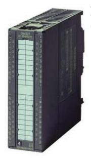
SIPLUS PCS 7 SM 321 16DI for medial exposure with conformal coating based on 6ES7321-7TH00-0AB0 . Digital "input ""16 DI; 24 V DC, 1x" "40-pole,"" diagnostics-capable," for contacts (wired/ not wired), NAMUR encoder, 3/4-wire "BERO, with chatter ""monitoring;" "Pulse"" extension, Open-circuit" detection Connection IM 153-2 required
