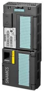
SIPLUS G120 CU240E-2 PN Control Unit CU240E-2 PN -20...+55°C with conformal coating based on 6SL3244-0BB12-1FA0 . E-type with Safety Integrated STO PROFINET 6DI, 3DO, 2 AI, 2 AO, max. 1F-DI PTC/KTY interface USB and SD/MMC interface Degree of protection IP20 without Power Module
