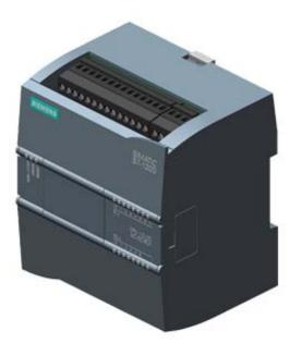
SIPLUS S7-1200 CPU 1212C AC/DC/relay -40...+70°C with conformal coating based on 6ES7212-1BE40-0XB0 . compact CPU, AC/DC/relay, onboard I/O: 8 DI 24 V DC 6 DO relay 2 A 2 AI 0-10 V DC, Power supply: 85-264 V AC at 47-63 Hz, Program/data memory 75 KB
