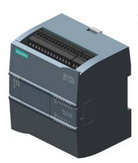
SIPLUS S7-1200 CPU 1212C DC/DC/DC -40...+70°C with conformal coating based on 6ES7212-1AE40-0XB0 . compact "CPU, DC/DC/DC, onboard I/O: ""8" "DI 24 V DC;"" ""6 DO 24 V DC;"" 2" AI 0-10 V DC, Power supply: 20.4-28.8V DC, Program/data memory 75 KB
