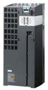
SIPLUS G120 PM 240-2 FSC 15kW Power Module PM 240-2 unfiltered -20...+50°C with conformal coating based on 6SL3210-1PE23-3UL0 . with integrated braking chopper 380-480 V 3 AC +10/-10% 47-63 Hz Power high overload: 11kW at 200% 3s,150% 57s,100% 240s Power low overload: 15kW at 150% 3s,110% 57s,100% 240s 355x 140x 165 (HxWxD), FSC Degree of protection IP20 without Control Unit and operating unit Released as of firmware version V4.6
