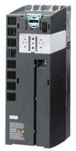
SIPLUS G120 PM 240-2 FSB 7.5kW Power Module PM 240-2 unfilt. -20...+50°C with conformal coating based on 6SL3210-1PE21-8UL0 . with integrated braking chopper 380-480 V 3 AC +10/-10% 47-63 Hz Power high overload: 5.5kW at 200% 3s,150% 57s,100% 240s Power rating low overload: 7.5 kW at 150% 3s,110% 57s,100% 240s 291x 100x 165 (HxWxD), FSB Degree of protection IP20 without Control Unit and operating unit Released as of firmware version V4.6
