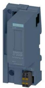
SIPLUS ET 200SP IM155-6PN HF -40...+60 °C with conformal coating based on 6ES7155-6AU01-0CN0 . 2-port interface module IM155-6PN/2 High Feature, 1 slot for BusAdapter, max. 64 I/O modules and 16 ET 200AL modules, S2 redundancy, multi-hot swap, 0.25 ms, isochronous mode, optional PN strain relief, including server module
