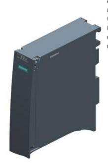
SIPLUS ET 200MP IM 155-5 PN HF -40...+60 °C With conformal coating based on 6ES7155-5AA00-0AC0 . PROFINET IO device interface module IM 155-5 PN HF, for ET 200MP electronic modules; Up to 12 IO modules without PS; Up to 30 IO modules with additional PS; Integrated 2-port switch; RJ45 shared device; MRP; IRT >=0.25 ms; Isochronous mode FW update; IM0...3; Prioritized run-up S2 redundancy; Shared device with 4 controllers
