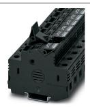
Fuse modular terminal block, fuse type: Glass / ceramics / ..., connection method: Screw connection, cross section:  $1.5 \text{ mm}^2$ -  $25 \text{ mm}^2$ , AWG: 16 - 4, nominal current: 32 A, nom. voltage: 690 V, width: 18 mm, fuse type:  $10.3 \times 38 \text{ mm}$ , mounting type: NS 35/7,5, NS 35/15, color: black
