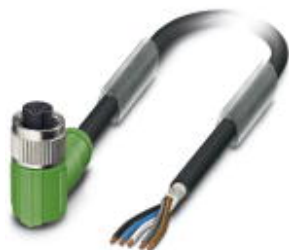
Sensor/actuator cable, 5-position, PUR halogen-free, black-gray RAL 7021, shielded, free cable end, on Socket angled M12, coding: A, cable length: 3 m
