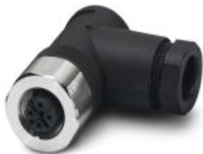
Connector, 5-position, Socket angled M12, Coding: A, Screw connection, knurl material: Stainless steel 1.4404, cable gland Pg9, external cable diameter 6 mm ... 8 mm
