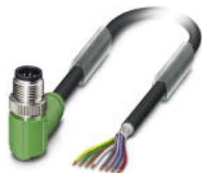
Sensor/actuator cable, 8-position, PUR halogen-free, black-gray RAL 7021, shielded, Plug angled M12, coding: A, on free cable end, cable length: 3 m
