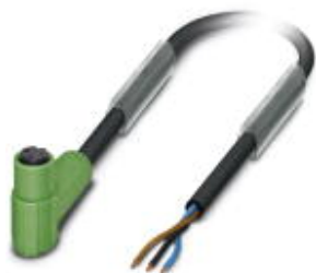
Sensor/actuator cable, 3-position, PUR halogen-free, black-gray RAL 7021, free cable end, on Socket angled M8 Snap-in, cable length: 5 m
