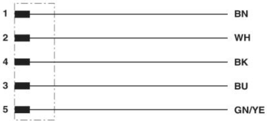
Contact assignment of the M12 plug
