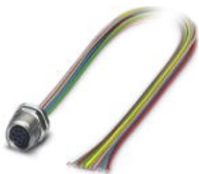
Flush-type connector, 8-position, Socket, straight, M8, Rear mounting, M10, Individual wires, cable length: 0.5 m, 0.14 mm 2 , PVC litz wire
