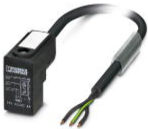
Sensor/actuator cable, 3-position, PVC, black RAL 9005, free cable end, on Valve connector C (8 mm), with 1 LED, connected with Varistor, cable length: 3 m
