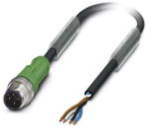
Sensor/actuator cable, 4-position, PVC, black RAL 9005, Plug straight M12, coding: A, on free cable end, cable length: 5 m
